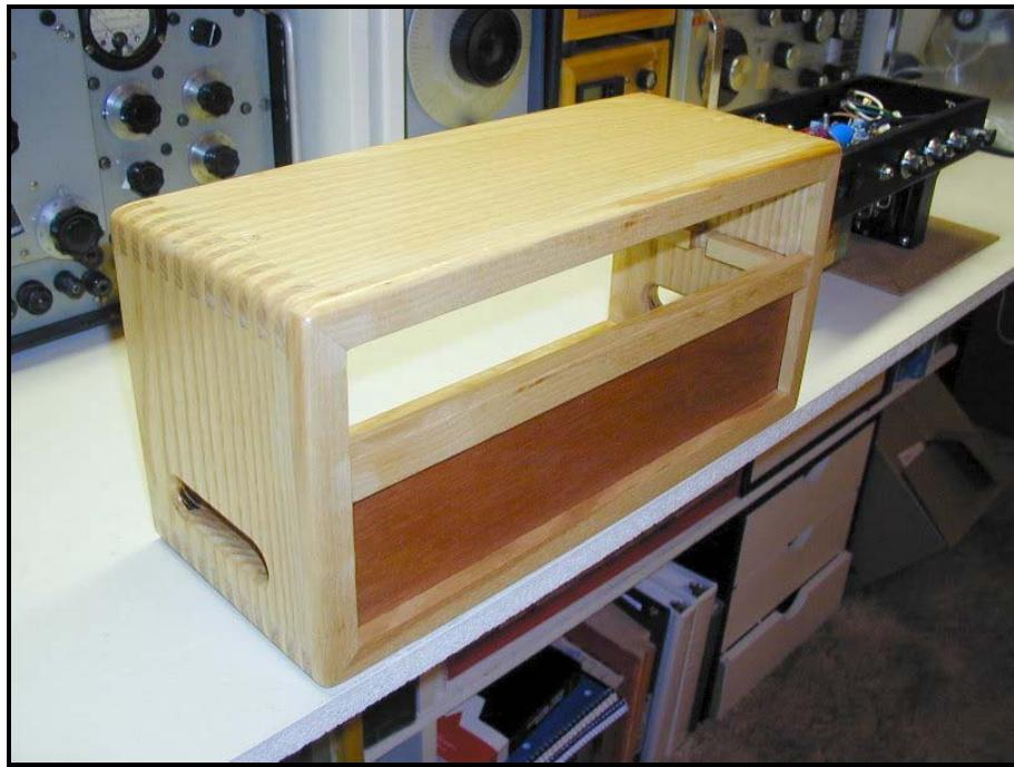
Note that to maintain the clean lines of the design, this cabinet has hand holes routed in the side instead of a standard handle secured to the top. (The hand holes also permit the circulation of cooling air within the cabinet.) The lower front panel of the enclosure is a small sheet of 1/4 inch mahogany plywood - the type is not critical.
