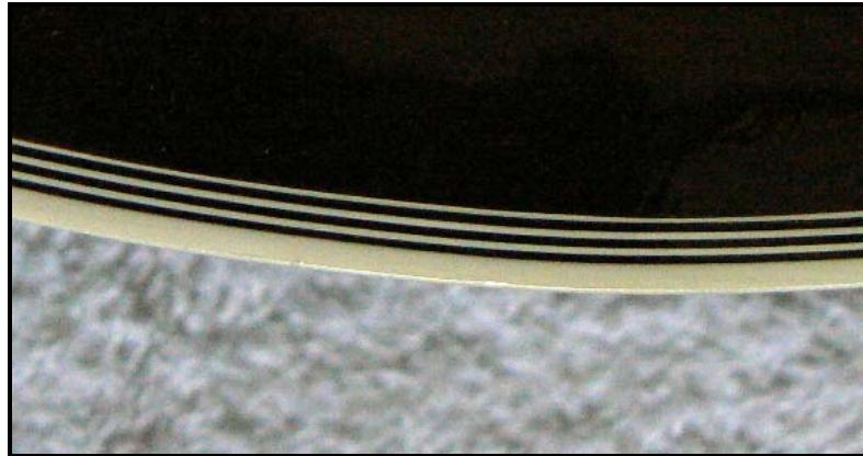
Five and seven-ply body bindings were common in top-grade professional instruments while single, two and three-ply bindings decorated workman-level instruments. Neck bindings were typically limited to a single ply material except for the higher cost guitars which were decorated with three to five-ply bindings, sometimes incorporating a "sculpted" appearance at the end of the neck like this L-5CES (note the five-ply binding on both neck and pickguard):
