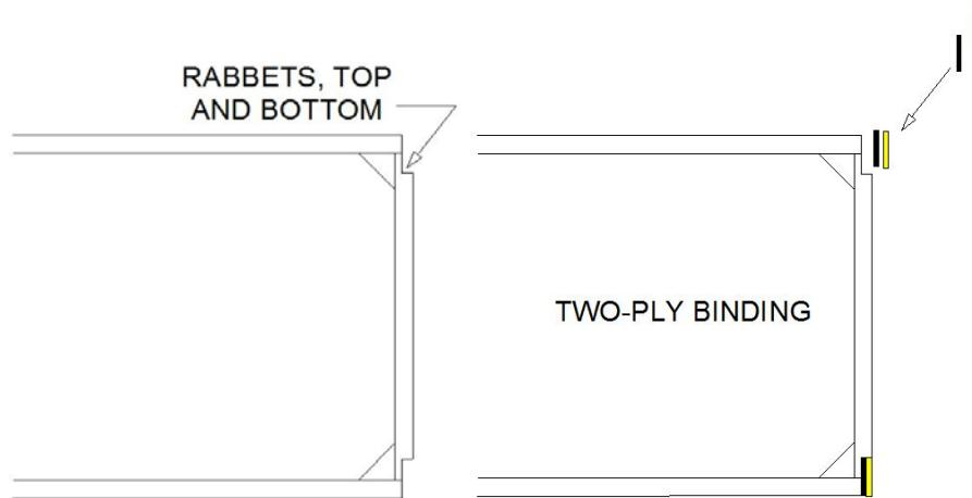
As shown in the second sketch, the binding is glued into the rabbets at the top and bottom of the guitar. The thickness of the individual binding strips is determined by the desired number of plies and the rabbet dimensions.
